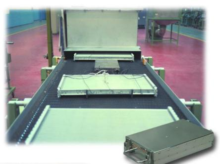
In slab re-heat furnaces, it is vital to ensure that the slab is at the correct rolling temperature throughout its thickness.
