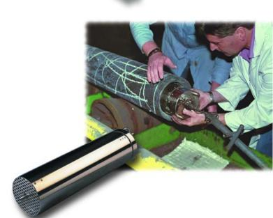
Use a Datapaq system in aluminium brazing applications where it is important to ensure the correct brazing temperature is achieved but not exceeded.
